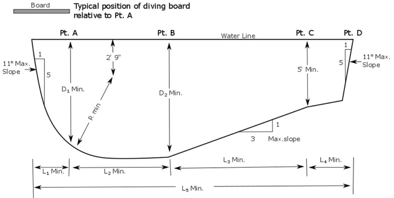
Note:  $L_4$  is a minimum dimension to allow sufficient length opposite the board. This may of course be lengthened to form the shallow portion of the pool.
