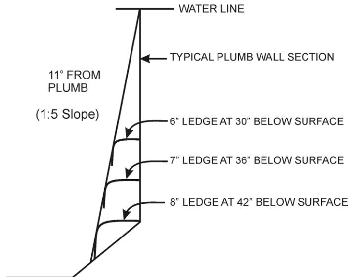
(9) **Underwater Seat Benches.** Underwater seat benches in pools, if provided, shall have a maximum horizontal seat bench depth of twenty inches below the waterline, be
